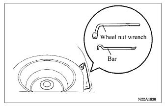
7. Remove the wheel nut wrench and bar from the tool bag (located inside the trunk).
